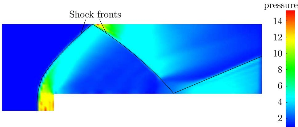
Figure 3.8: Shock fronts in the forward step problem
