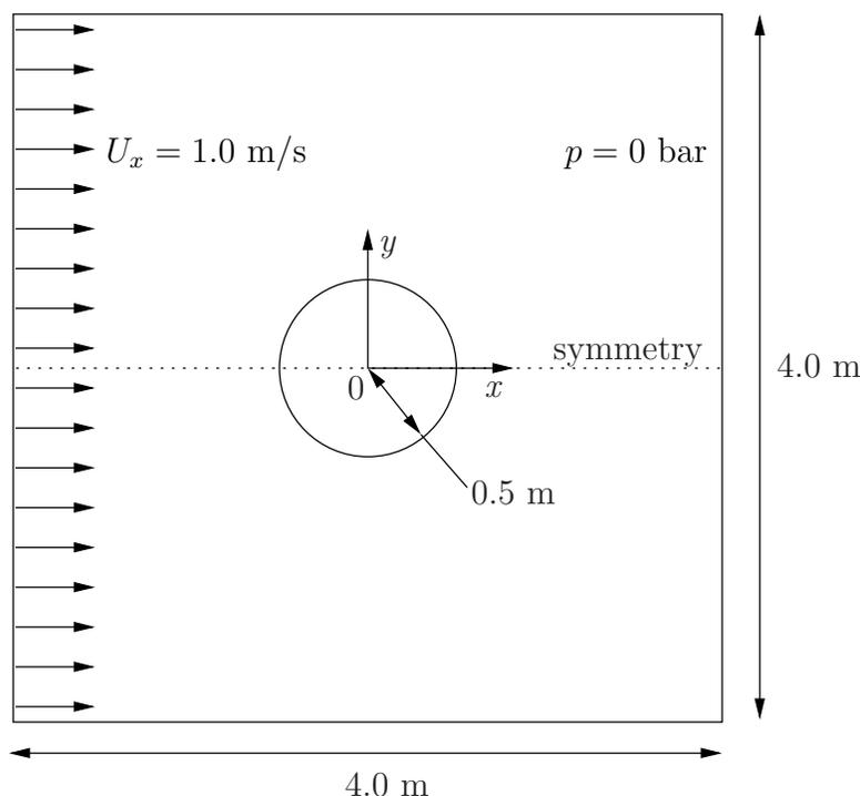
Figure 3.1: Geometry of flow round a cylinder
