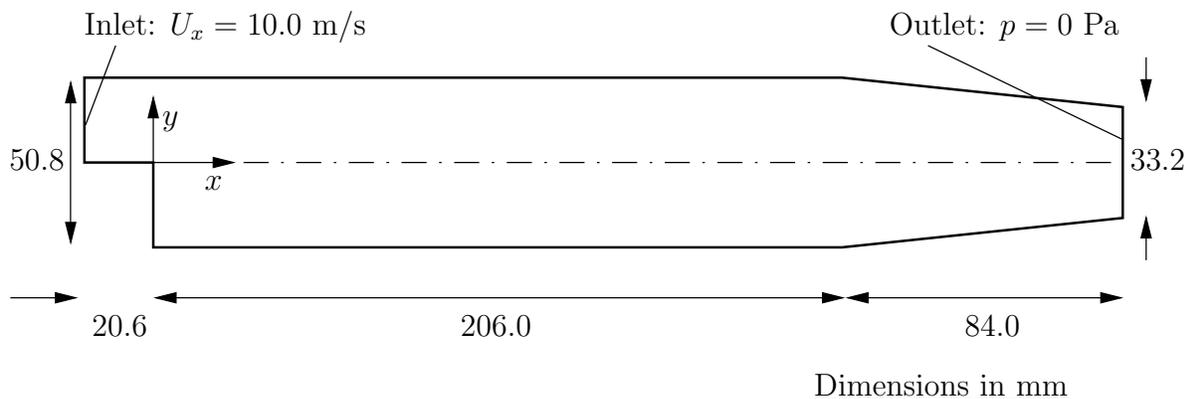
Figure 3.4: Geometry of backward-facing step
