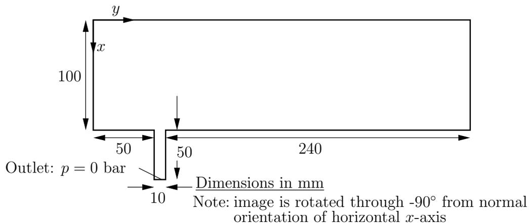
Figure 3.9: Geometry of a tank with outflow pipe
