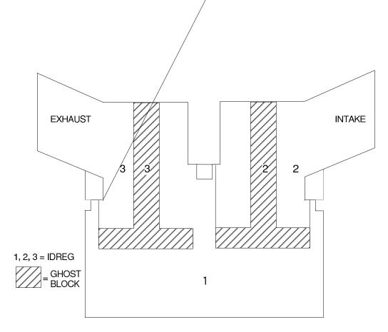
Fig. 1. The three physical regions in a KIVA-3V grid for a typical valved IC engine.
