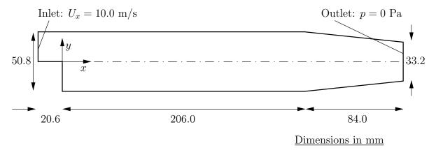
Figure 3.4: Geometry of backward-facing step
